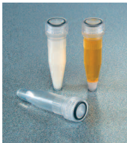
Fig 2. The effect of the StatSpin LipoClear system on a lipaemic sample, showing the clearing achieved (right) after centrifugation.
